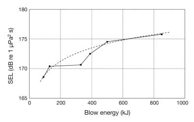
Fig. 5. Broadband sound level as a function of pile driver blow energy, observed at 720 m distance. The formula of the fitted dashed curve is SEL = 7.5 log(E) + 154. Each point represents the energetic average from between 10 and 26 blows, depending on the energy level. SEL: singlestroke sound exposure level
