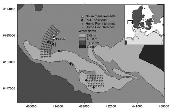
Fig. 1. Study area. Positions of the wind turbines of the windfarm Horns Rev II, where pile driving took place during this study (●), and the windfarm Horns Rev I (▲) that was already installed. ● 1 to 6 = positions of the T-PODs. □ = positions where noise measurements were conducted during pile driving of monopile J2 (O). Grid reference system is UTM 32 N
